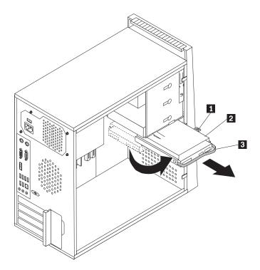
Figure 21. Removing the primary hard disk drive
